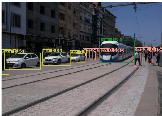
Figure 4 Example of Road object detection and recognition result for an image of Algiers obtained by our model optimized.
